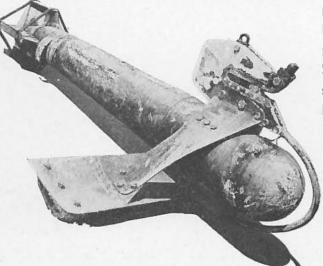
paravane the mine mooring is severed by a cutter. The picture to the left is of a United States paravane, and clearly shows the cutter on top of the float. The sketch to the right illustrates the progressive steps in the catching of a mine by a bow paravane.
