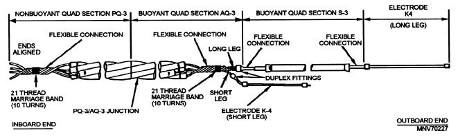
Figure 10-1.—Magnetic quadded tail assembly.
