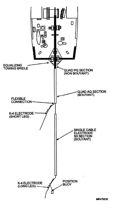
Figure 10-6.—Magnetic sweep cable configuration M Mk 5 (a).
